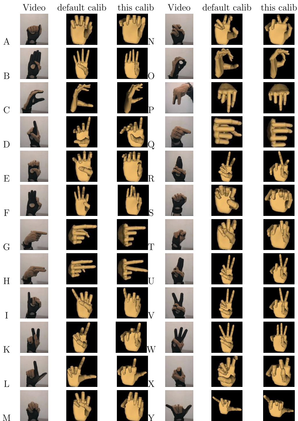
Figure A.2: Rendering of the hand using the “default” calibration (provided with the CyberGlove) and the calibration presented in this section, for the static fingerspelling alphabet of American Sign Language. The letters that require movement (J and Z) are not shown.
